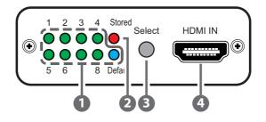
LED indicators 1~8: When in Stored or Default mode, each of these LEDs indicate a different EDID setting (1 to 8). Press the 'Select' button to switch between settings, the LED will illuminate to indicate the current selected settings. For the default EDID settings, please refer to section 6.3 - Factory Default EDIDs.
