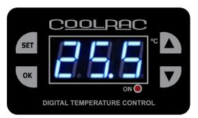
**PLEASE NOTE:** The temperature probe must be plugged in for this unit to operate, an alarm will sound if it is not connected.
