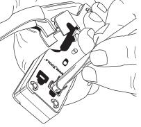
6) Roll up the drain wire and place in the base of the external ground. As you start to bring the external ground into place onto the cable, keep the mass of drain wire tucked in so it is totally covered.
