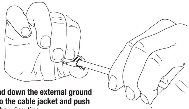
Bend down the external ground onto the cable jacket and push in the wing tips.
