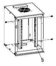
(2) Secure the top panel, bottom panel and side panels using 4pcs M4x8 self-tapping screws at the four corners in the front of the cabinet.
