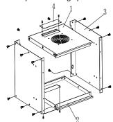
(3) Fit the vertical mounting rails in the desired position using 4pcs M5x12 pan head screws.
