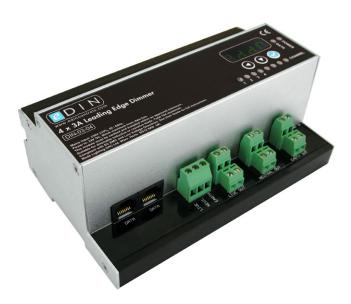
A four circuit dimmer module rated at 700W per circuit for the control of resistive and inductive lighting loads with the facility to select dimming or switched only operation of any circuit. A custom designed housing provides reliable power handling in a compact format.
