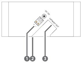
**DC 12V Port:** Plug the 12V DC power adapter into this terminal block and connect it to an AC wall outlet for power. (Optional)
