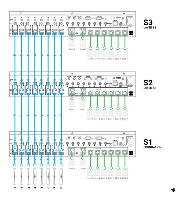
Video sources (1-8) are connected to the Foundation Layer (S1) and <u>Connections</u> have been defined in uOS connecting the "Mirror (Out)" ports on (S1) to the "Source (IN)" ports on (S2) for all 8 ports. This is repeated again on (S3).
