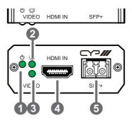
Power (の) LED: This LED will illuminate to indicate the unit is on and receiving power.
