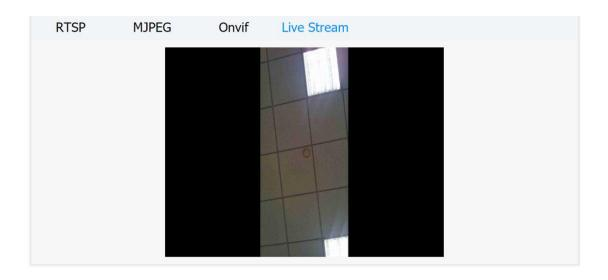
To check the real time video using URL, you can enter the correct URL (http://IP\_address:8080/video.cgi) on the web browser if you want to obtain the real-time video directly with going to the web interface.
