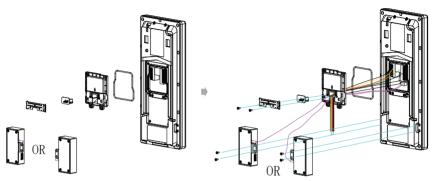
Take out the device and the digital wrist temperature detector and then take out wiring cover, sealing pressing plate, rubber plug, sealing ring and corresponding screws.
