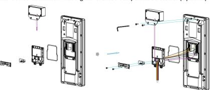
Take out the device and the digital forehead temperature detector and then take out wiring cover, sealing pressing plate, rubber plug, sealing ring and corresponding screws.
