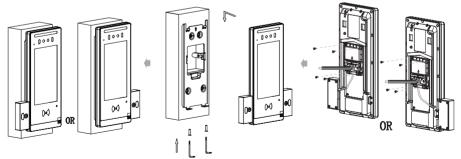
Installation is completed. And please remove the protective film.
