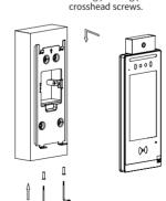
Hang the device on to the square hanger on the wall mounting bracket, Installation is completed. pull down the device to make it fall completely on to the square hanger on the wall-mounting bracket, then use the torx wrench attached to tighten the device with 2 M3x9.5 torx head screw.
