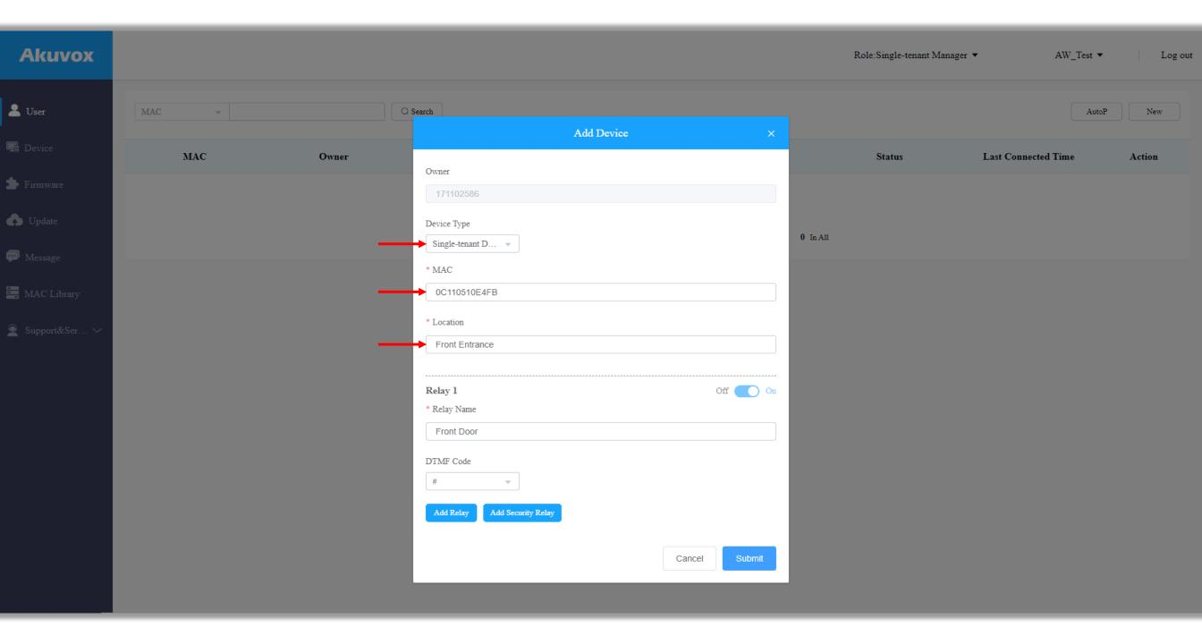
Enter the MAC address of the door intercom, select 'Single-tenant Doorphone' as the Device Type and enter the location of the intercom. The location name given will be visible to the end user in the SmartPlus app so make it logical and familiar to the user.
