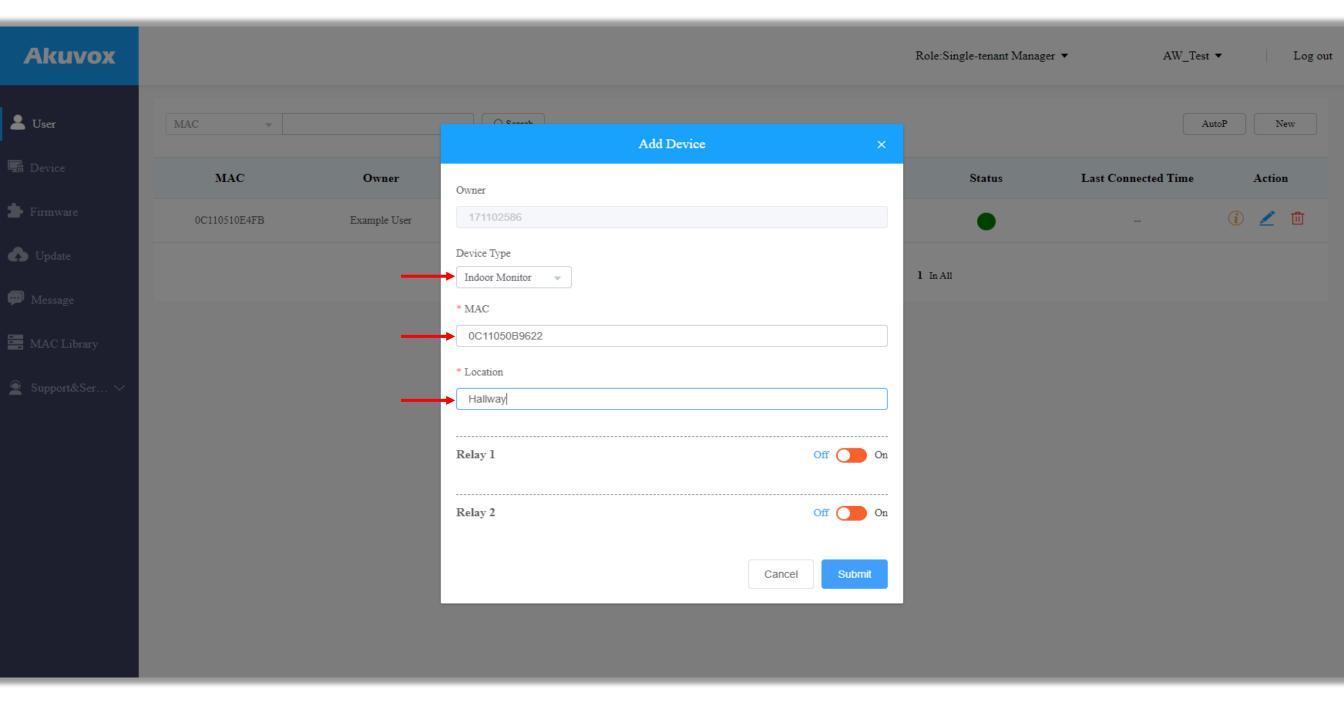
Fill in the MAC address of the indoor monitor, but this time select 'Indoor Monitor' as the Device Type. Once again, make sure that you give the device a logical location name relevant to where the device has been installed within the property. Click 'Submit' when ready.
