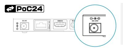
Ability to connect a single PSU to either transmitter or receiver adding extra convenience to your install. 24V PoC is standardardised accross all Netvio HDBaseT products.
