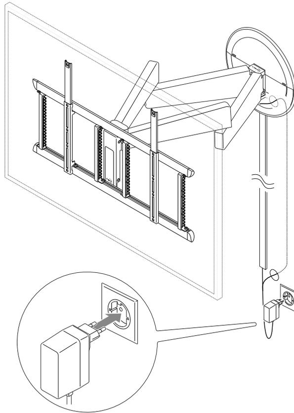
7. Connect the **power cable** (V) to the power outlet.
