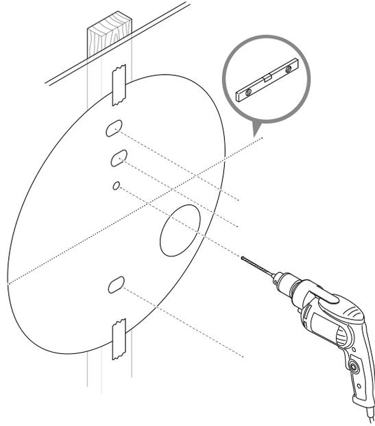
2. Now for the fun part... drilling the holes. Make sure to drill the positioning hole first.
