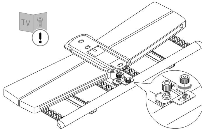
2. Remove the **thumbnut** and detach the **wall mount** ① from the **interface**. Keep the **thumbnut** for later use.
