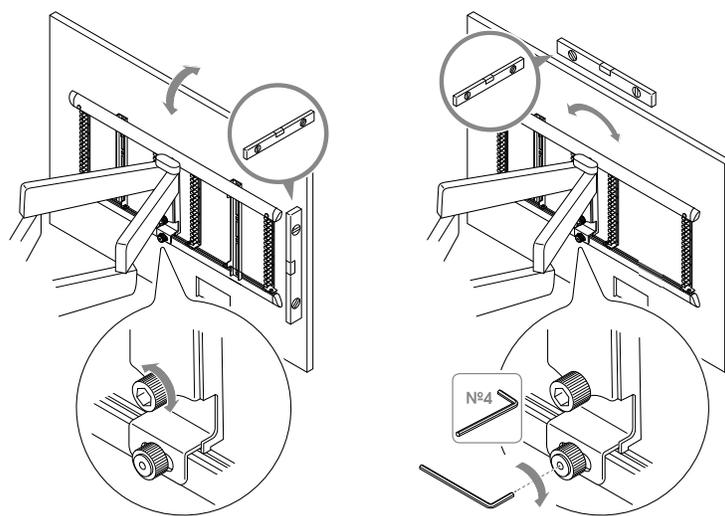
3. Level the **wall mount** and the TV screen. Use a spirit level and the **Allen key** to correct the position. Tighten the **thumbnut** and the **thumb bolt** with the **Allen key** when finished.
