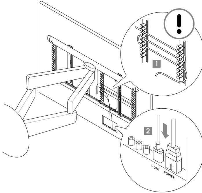
5. Connect the power cable and the **HDMI 2.0 (2 meter) cable** to the TV. Make sure all other cables are neatly stowed away by using the vertical cable clip strips on the **interface**.
