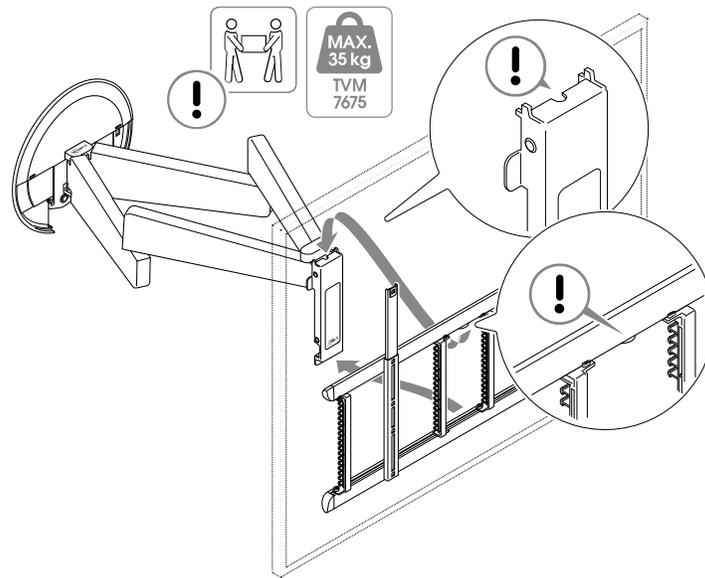
1. Carefully lift and attach the TV onto the interface bracket on the **wall mount** ④. Make sure the plug on the interface falls into the notch on the wall mount.
