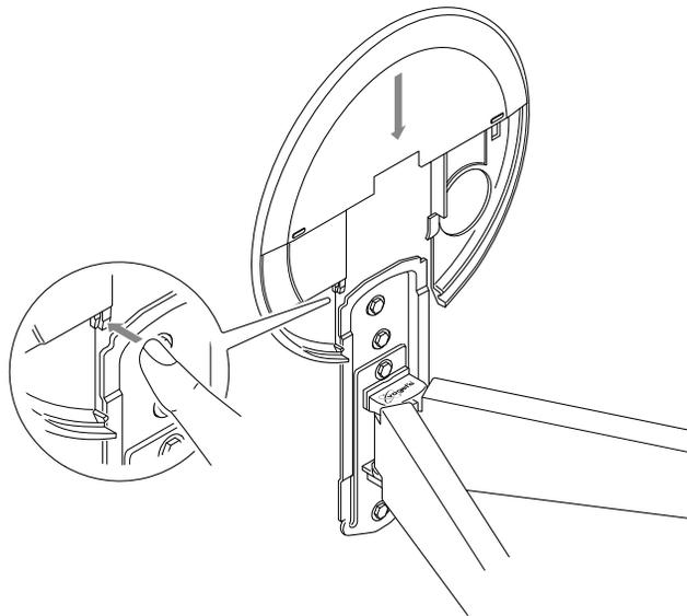
5. Slide the **wall plate cover** Ⓚ onto the **wall mount** Ⓐ. To remove the cover plate, press the left tab and slide it off the wall mount.
