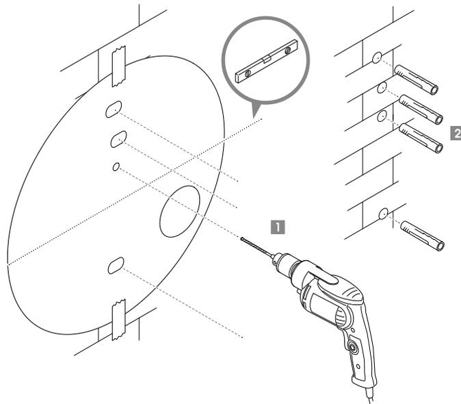
2. Drill the holes. Make sure to drill the positioning hole first. Pre-drill with a smaller drill to avoid damage to the wall.
