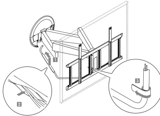
1. Attach the **cable sleeve** ① to the **wall mount** ②, by sliding it into the holes on the bottom side of the right arm.
