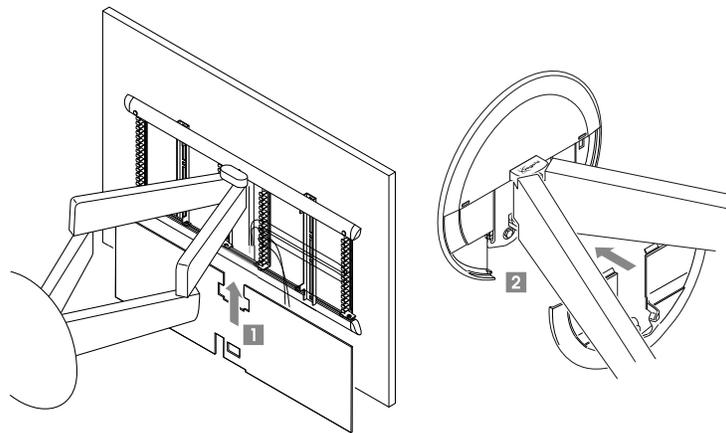
6. Put the **wall plate cover** (K) onto the wall mount and the **interface cover** (Y) onto the back of the **interface**.
