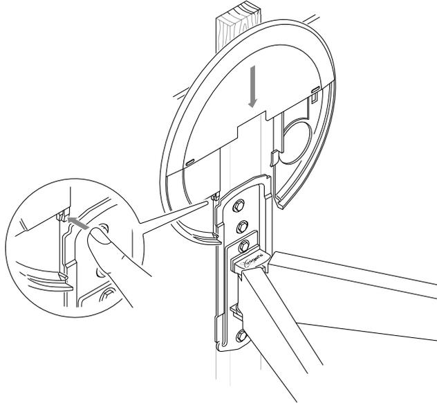
4. Slide the **wall plate cover** (K) onto the **wall mount** (A). To remove the cover plate, press the left tab and slide it off the wall mount.
