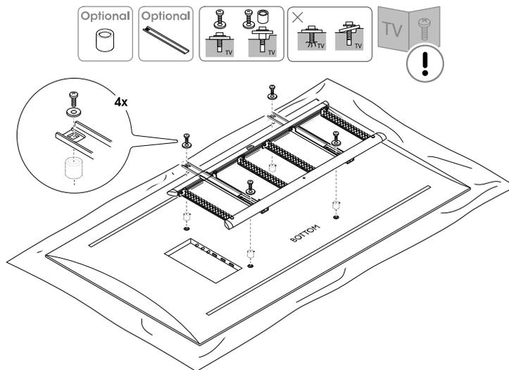
5. Attach the **interface** to the TV screen with the **bolts** ⑤ and **spacers** ⑥. Make sure the top side of the frame is positioned correctly, as indicated by the word 'top' on the **interface**.
